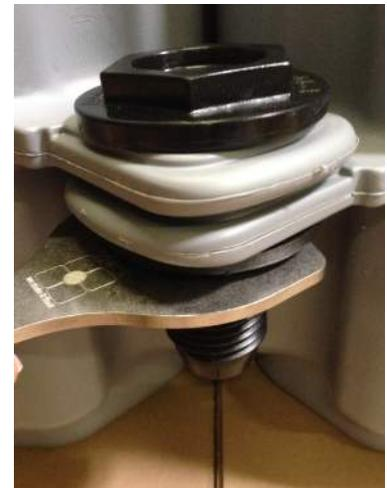
9. For each connection you need a lug connector (SKU 3312) and a nut (SKU 3273). Insert the lug connector through the lugs and tighten by hand.
