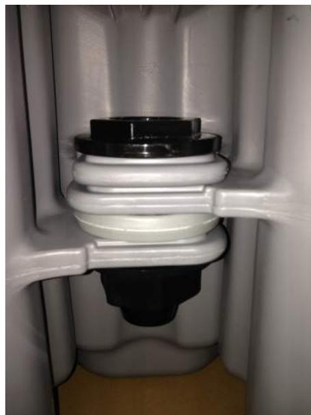
10. For convenience, if you have a lot of joints to tighten, you may wish to obtain from us a 60mm socket & a  $\frac{3}{4}$  -  $\frac{1}{2}$ " socket converter which fits a standard socket set ratchet. To tighten them you can also use the standard tool for lug connector (TL-003) as shown above (p.5).
