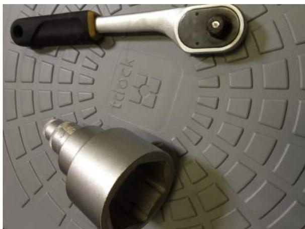
11. Then, after you have launched and installed your pontoon, go back and re tighten all the connecting pins (SKU 3380) firmly with the tool (TL-001).
